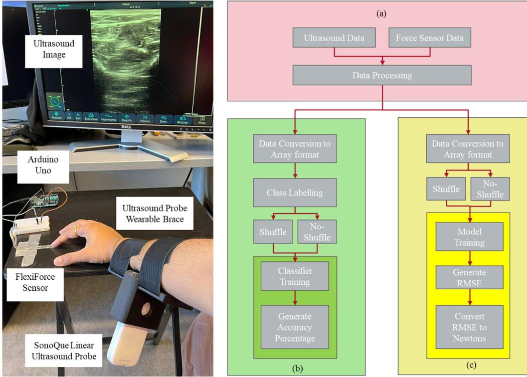
Fig. 1. System components and workflow: (a) The data acquisition block, (b) The classification block, (c) The continuous estimation block.
