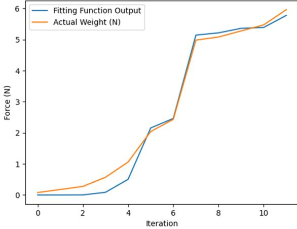
Fig. 2. Force sensor calibration using a quadratic fit function
